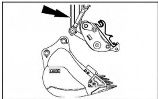
5. Operate the arm and bucket controls so as to bring the quick coupler hook (2) around the attachment pin (3).
